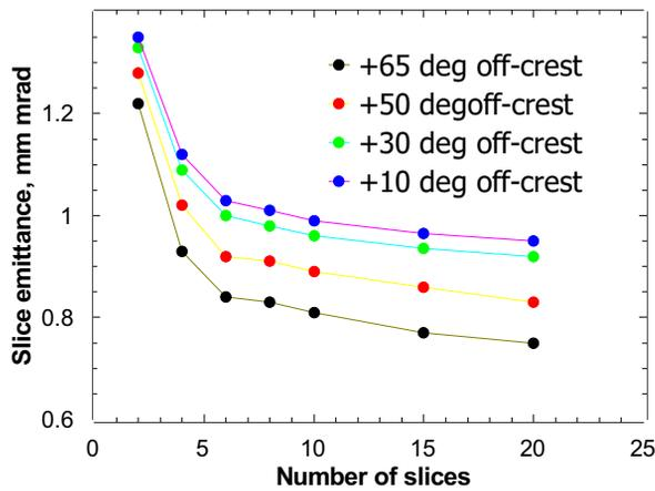
Figure 3: Slice emittance saturation at about 1ps resolution. The slice emittance is smallest at the waist position. The converging beam waist position depends on the off-crest phase
