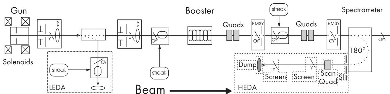
Figure 1: Part of PITZ facility up to the first high energy dispersive section.
