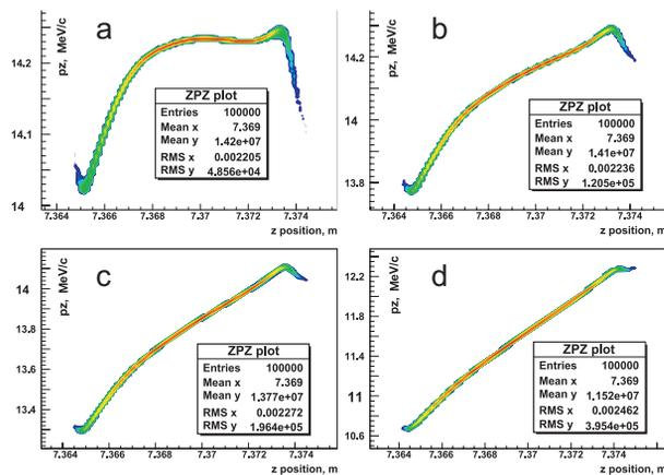
Figure 2: Longitudinal phase space after the booster: a) on-crest; b) +10 deg; c) +30 deg; d) +50 deg.
