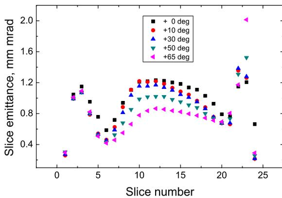
Figure 4: Simulated slice emittance of the beams accelerated with different phases off-crest.
