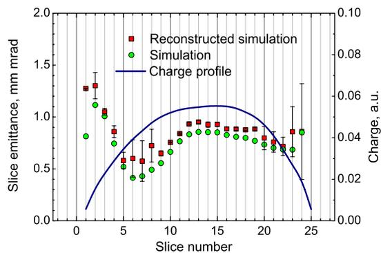
Figure 6: Simulated slice emittance measurement at +65 deg off-crest. Temporal resolution is 0.8 ps
