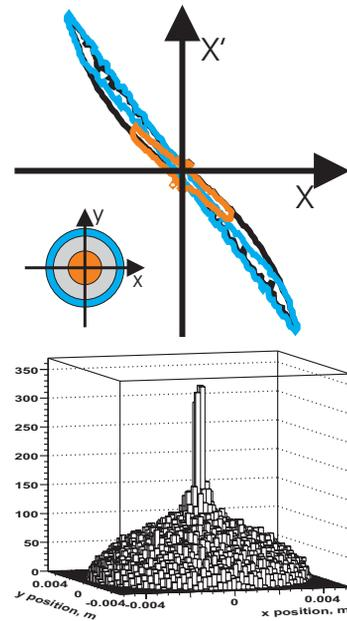
Figure 5: The non linear space charge force separates the phase space ellipses of the central(orange) and the periphery(blue) parts of the transverse profile.
