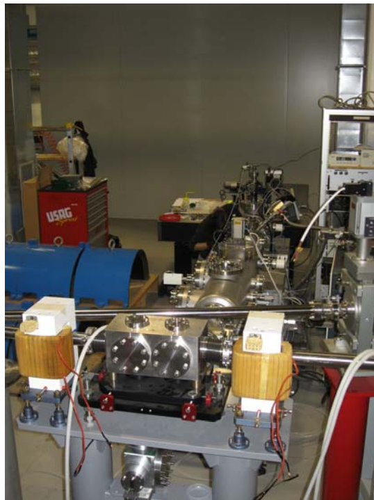
Figure 1: Detail of the magnetic chicane and of the injection periscope for the seeding experiment at SPARC.
