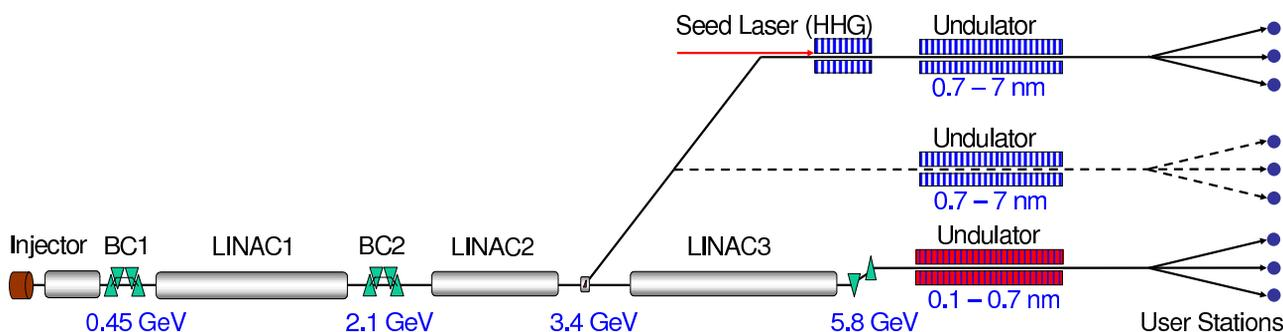
Figure 1: Schematic layout of the SwissFEL facility.
