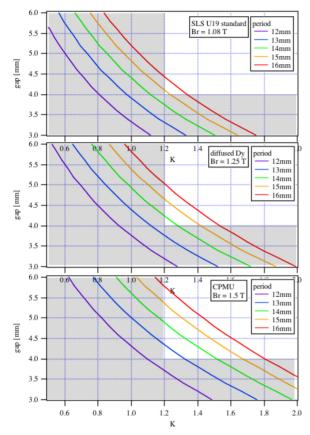
Figure 9: Gap versus K value for period length between 12 and 16 mm. The three graphs differ in the remanence of the magnets.
