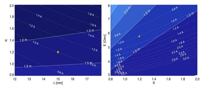
Figure 3: SwissFEL hard x-ray undulator working point. Optimization based on the Ming Xie model [7]. The plots show the gain length for various wavelength around 1Å due to variations of period, K and electron energy.
