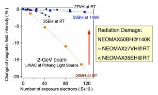
Figure 5: Degradation of various NdFeB magnet types due to exposure with 2 GeV electrons. The degradation is strongly correlated with the coercivity. 27VH is the material used for the SLS U19 undulators. 50BH has lower coercivity at room temperature and shows large degradation. But cooled down to LN2 temperatures increases stability drastically (courtesy of T. Bizen, SPring-8).
