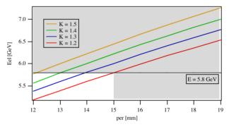
Figure 2: Possible periods and related K values to meet the specifications for the hard x-ray undulator With a maximum electron energy of 5.8 GeV and a minimum K value of 1.2 the maximum allowed period length is 15 mm. All possible options are in the white area at the left bottom side.
