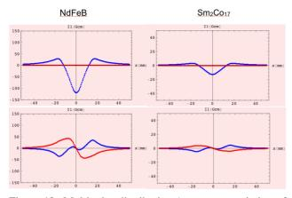
Figure 10: Multipoles distribution (transverse variation of the first field integrals or kicks) due to nonlinearity of the permanent magnet material in circular and linear mode for NdFeB and  $Sm_2Co_{17}$ .
