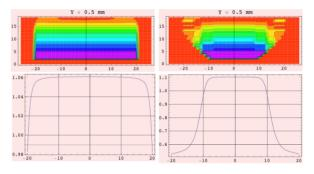
Figure 8: Field optimization by optimized pole profile.
