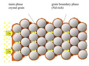
Figure 7: Increased coercivity of NdFeB magnets by diffusion of Dy into the ready made magnet. The Dy concentrates only at the grain boundaries (courtesy of Hitachi Metals Ltd.).
