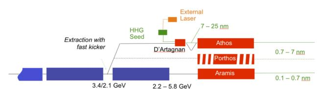
Figure 1: SwissFEL undulator concept: two soft x-ray undulators with variable gap can be served by 2.1 or 3.4 GeV electron energy, the hard x-ray line will be tuned mainly by electron energy variation. Seeding in the soft x-ray is envisaged as well.
