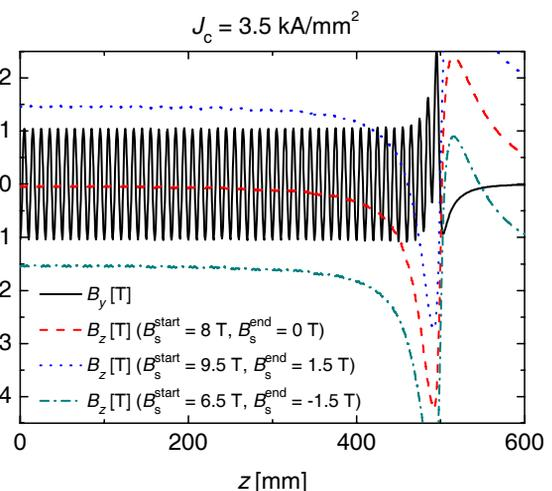
Figure 7: Basically the same with Fig. 8. The solenoid field at the end of the magnetization process was  $B_s^{\text{end}}=+1.5, 0, -1.5$  T.  $B_z$  can be changed without  $B_y$  change.
