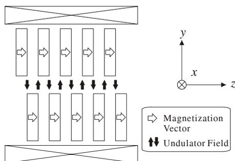
Figure 1: Schematic of new type undulator. White arrows indicate magnetization vectors of HTSC magnets. All magnetization vectors parallel to the direction of  $+z$ . Black arrows indicate undulator fields.
