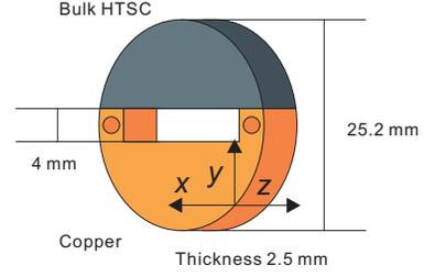
Figure 3: A bulk HTSC magnet and a copper piece (a half period).
