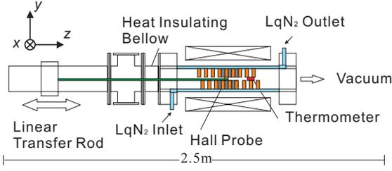
Figure 2: Experimental setup of 11 period prototype. The bulk HTSC magnets and the copper pieces (Fig. 3) are stacked in the vacuum chamber.
