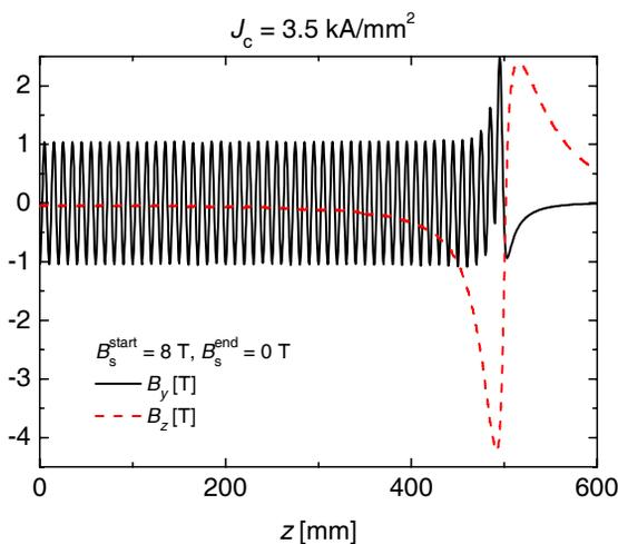
Figure 6: The distribution of the y and z-component of the magnetic field ( $B_y$  and  $B_z$ ) along  $z$  axis in Bulk HTSC SAU.
