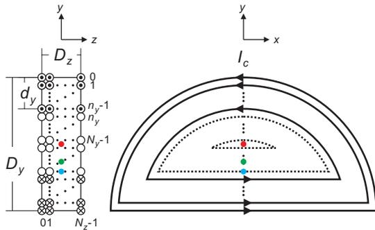
Figure 4: Numerical model of bulk HTSC magnet. The bulk represented by  $N_y$  times  $N_z$  line loop currents. The red point indicates the centre of bulk ( $D_y/2, D_z/2$ ).
