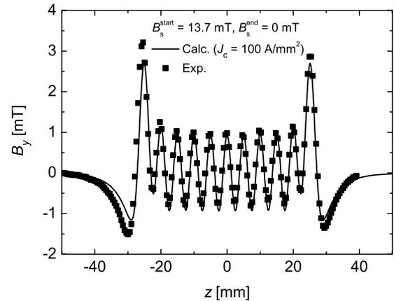
Figure 5: The comparison between the calculation and the experiment. The field distribution of the experiment was well reproduced by the calculation without the edge.
