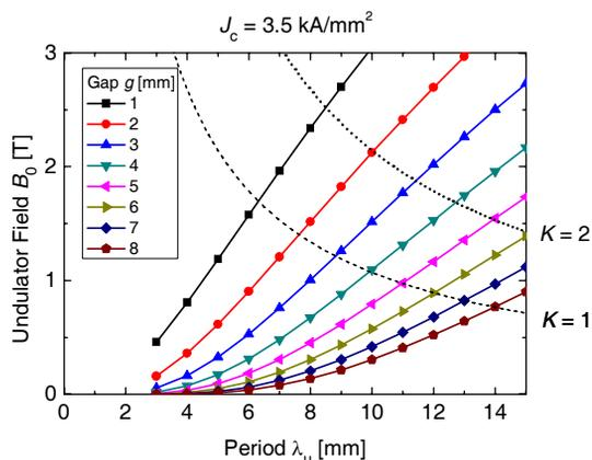
Figure 8: The undulator field dependence on the period and the gap of Bulk HTSC SAU. We assume the critical current density of 3.5 kA/mm<sup>2</sup>.
