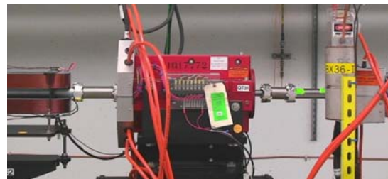
Figure 2: LTU beam line: corrector, bellows, quad, chamber step and bellows.
