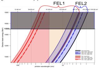
Figure 2: Tuning ranges for both FERMI FELs for different electron beam energies. While FEL-1 has a large wavelength tunability at fixed energy (due to the 55-mm undulator period), FEL-2 tunability at fixed energy is limited by the 35-mm final radiator period to about +/-10% in the case of vertical polarization.
