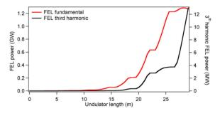
Figure 4: Results of numerical simulation of FEL-2 operating at 4.2nm in horizontal polarization.
