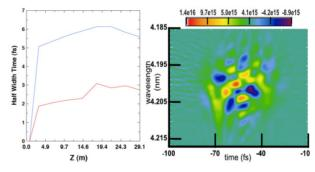
Figure 8: (a) Evolution of the coherence length of the FEL pulse at 4.2 nm along the final radiator. (b) A Wigner transformation of the far field, on-axis, complex FEL electromagnetic field.
