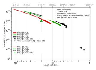
Figure 3: Expected output levels (photons/pulse) for the two FERMI FEL's. Solid lines: estimates using adaptation of M. Xie scaling formula [5] to adjust for increased energy spread in final radiator. Points: results of start-toend numerical simulation (GPT + ELEGANT + GINGER/GENESIS).
