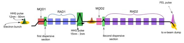
Figure 9: The same layout used for the double cascade scheme may be used without modification for implementing a HHG-seeded FEL, including both HGHG and direct amplifier configurations.
