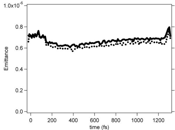
Figure 4: Electron-beam horizontal (full line) and vertical (dotted line) emittance profiles.
