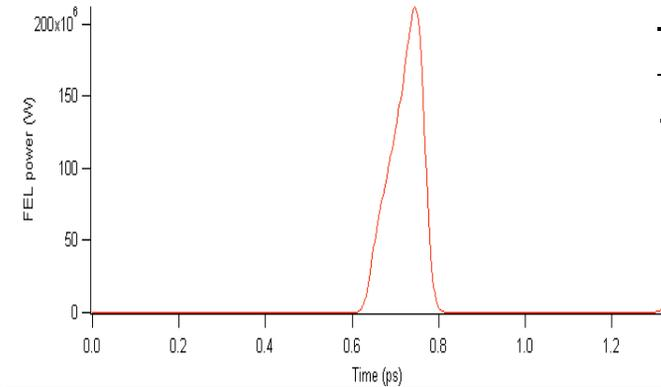
Figure 10: HGHG pulse at 60 nm.
