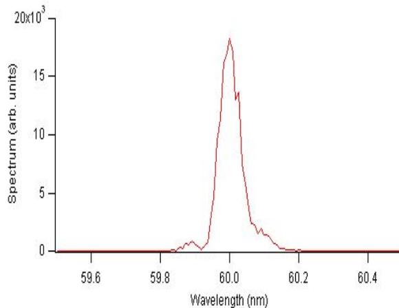
Figure 11: HGHG spectrum at 60 nm.
