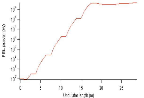
Figure 6: SASE power at 60 nm as a function of the undulator distance. For the simulation, we used the beam parameters corresponding to half-height of the current spike shown in Figure 3, that is: energy: 1.22 GeV, energy spread: 300 keV, current: 900 A, emittance: 0.7 mm mrad.
