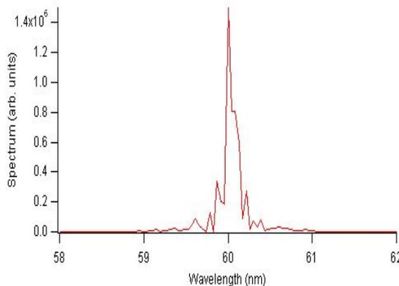
Figure 8: SASE spectrum at 60 nm.
