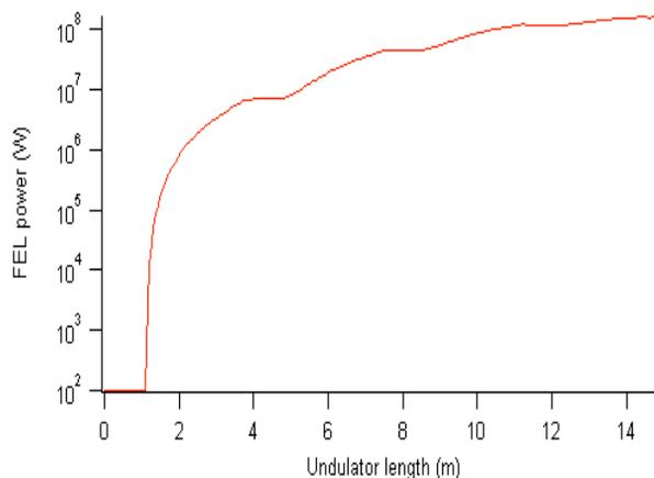
Figure 9: HGFG power at 60 nm as a function of the radiator length. For the simulation, we used the parameters corresponding to the center of the electron bunch (see figs. 2-5), i.e.: energy: 1.22 GeV, energy spread: 20 keV, current: 200 A, emittance: 0.7 mm mrad.
