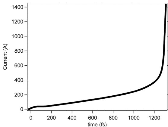
Figure 3: Electron-beam current profile.
