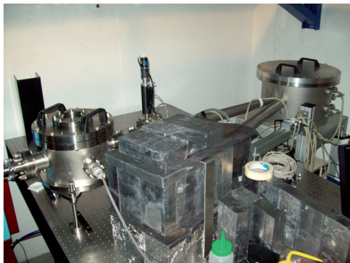
Figure 5: Undervacuum spectrometer installed at the end of the undulator.
