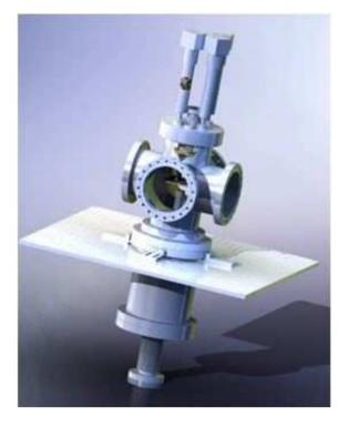
Figure 4: Diamond Field Emitter Cathode test stand
