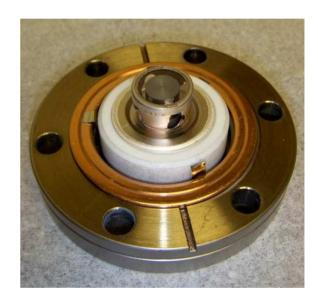
Figure 3: Dispenser Cathode example tested to determine level of material off-gassed into the vacuum
