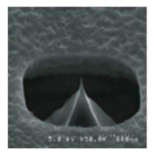
Figure 5: Single Diamond Field Emitter example
