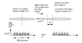
Figure 3: Sketch of principle of multi-color X-ray pulse generation in the baseline XFEL undulator. Here the SASE shutter is off. Modulation of the electron beam due to the FEL process in the first undulator part is washed out in the magnetic chicane. In the second part of the undulator, the seeded main part of electron bunch reaches saturation with ten GW power level at 0.2 nm wavelength.
