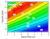
Figure 5: Variation in emittance (mm-mrad) at 300 MeV as function of choice of Twiss parameters at injection.
