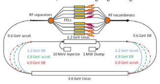
Figure 7: A ~10 GeV "GERBAL" multipass FEL driver; independent transport lines for each pass provide operational flexibility. RF separation/recombination of beams allows simultaneous service to several FELs.
