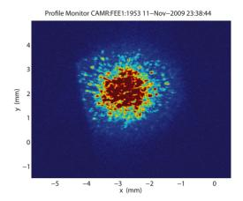
Figure 5: Image of the fundamental FEL signal following the third soft X-ray mirror. The sharp edge on the left side suggests the beam has been cut by an aperture. The speckle pattern is due to diffraction from a beryllium attenuator.
