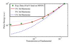
Figure 9: Measured pulse energy vs. gas attenuator strength. Measurement is for a fundamental photon energy of 8 keV, with fundamental pulse energy of 1.5 mJ, and corresponds to approximately 3% third harmonic.
