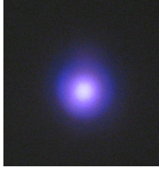
Figure 2: Spot of the 266nm radiation seed generated in gas as observed on a screen at about 15 m from the interaction point.
