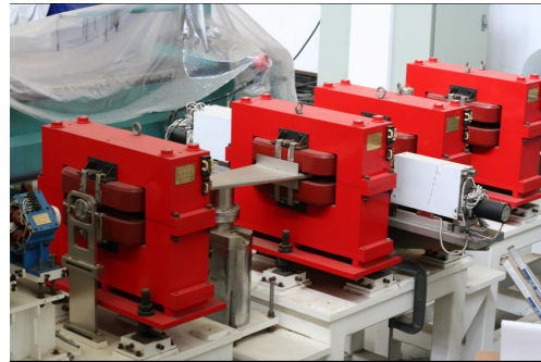
Figure 2: Bunch compressor of SDUV-FEL
