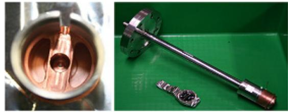
Figure 4: (a) New type RF coupler and (b) triode RF gun.
