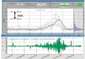
Figure 6: (Top) BC1 BAM acquisitions while klystron 3 phase was becoming temporarily instable (bottom). Total time window is roughly ten minutes.
