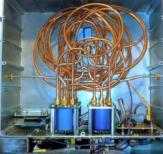
Figure 3: The programmable coaxial delay unit, nicknamed "spaghetti box", as it appears once the box is open; the origin of its name is quite obvious, at least in Italy.
