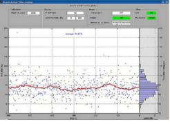
Figure 5: A 10 minutes continuous acquisition from the BAM station located downstream of BC1; each dot represents the rms value from 10 single shot acquisitions. The average value is 74fs.
