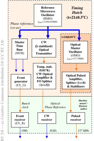
Figure 1: Basic block diagram of the FERMI@Elettra timing system. Blu lines indicate coaxial cables; orange lines, optical fibres. Temperature stability of the timing hutch and of individual systems is stabilized to 0.01°C.
