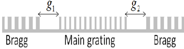
Figure 4: Schematic of Smith-Purcell free-electron laser with Bragg reflectors.
