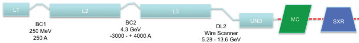
Figure 1: Schematic showing the linac section L2 where chirp is applied, the dispersion section DL2 where electron energy measurements were made; and the monochromator and spectrometer, where the spectral measurements were made.
