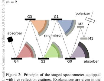
Figure 2: Principle of the staged spectrometer equipped with five reflection gratings. Explanations are given in the text. To avoid FIR absorption in humid air, the spectrometer is mounted in a vacuum vessel (not shown).
