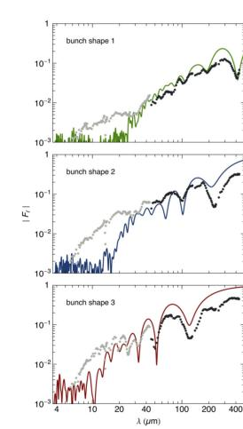
Figure 6: The magnitude  $|F_{\ell}(\lambda)|$  of the longitudinal form factors of the bunch shapes shown in Fig. 5. Solid curves: form factors computed by Fourier transformation from the longitudinal bunch profiles. Dotted curves: form factors derived from the spectroscopic measurements (black dots: FIR configuration, gray dots: MIR configuration).
