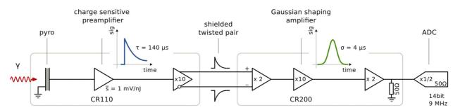
Figure 3: Electronics diagram. The preamplifier and the twisted-pair line driver amplifier are mounted on the electronics board inside the vacuum vessel. Line reciever, Gaussian shaping amplifier and ADC are located outside the the vacuum vessel.
