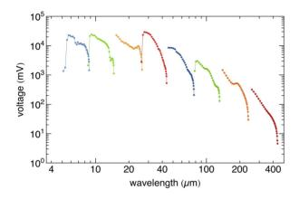
Figure 4: Computed overall response function of the multichannel spectrometer as installed at the CTR beamline at FLASH. The expected voltage in the ADCs is plotted as a function of wavelength. For details see text. The enhancement around 30  $\mu$ m is due to an enhanced pyroelectric detector sensitivity in this range.
