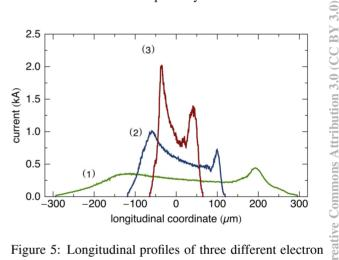
Figure 5: Longitudinal profiles of three different electron bunches in the FLASH linac as measured with the transverse deflecting microwave structure.
