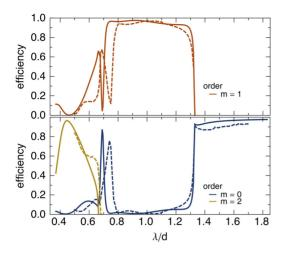
Figure 1: Efficiency curves of a gold-plated reflection grating for radiation polarized perpendicular to the grooves, computed with the codes PCGrate (solid curves) and GSolver (dashed curves). Top graph: first-order diffraction m = 1. Bottom graph: diffraction orders m = 0 and m=2.
