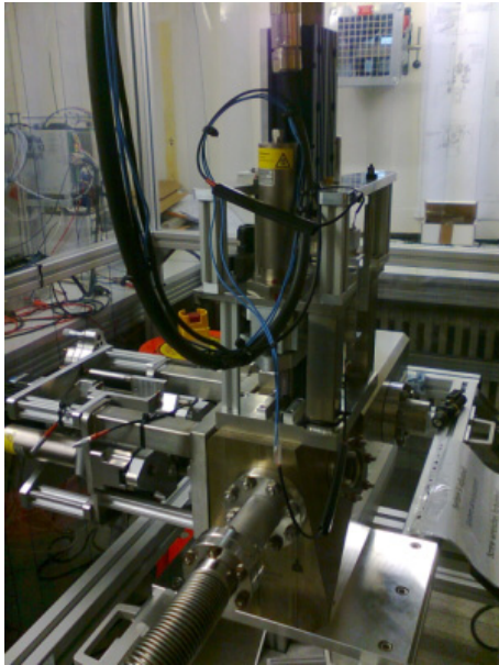
Figure 4: Picture of a vacuum chamber with mounted wire scanner.
