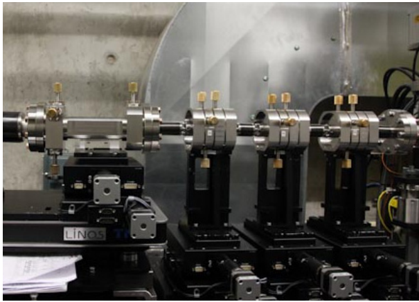
Figure 2: Picture of the cavity BPM teststand at FLASH. The beam enters from right to left. First 3 BPMs are for the undulator intersection, the last one is for the standard beamline.
