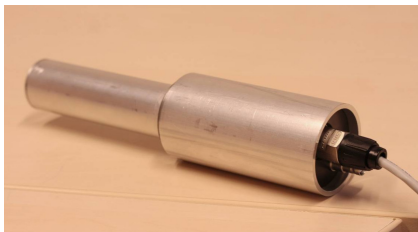
Figure 8: Picture of a scintillator with photomultiplier.
