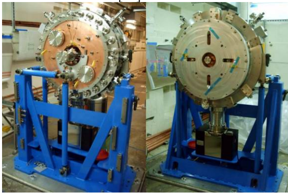
Figure 5: The VHF gun installed inside the BTF. The figure shows the gun back wall on the left, and the front wall with the beam exit port in the right.
