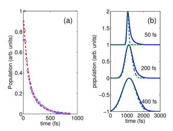
Figure 3: Monte-Carlo simulation (squares) taken from Ref. [13] and parametrization (dashed line) of the electron transit time from an initial Dirac-like laser excitation (a). Impact of the slow response time on the photoemission profile (blue traces) for three different Gaussian-like laser profiles (green dashed traces) of indicated rms duration (b).
