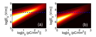
Figure 1: Domain of existence of the blow-out regime (lighter colors) in the  $(\sigma_0, E_0)$  parameter space for  $\tau_l = 50$  fs (a) and  $\tau_l = 200$  fs (b). The horizontal blue dashed lines correspond to  $E_0 = 35$  MV/m.
