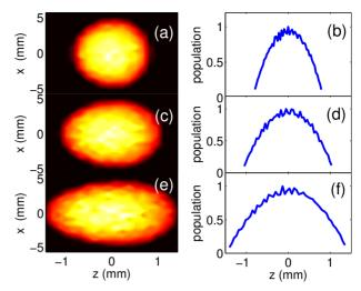
Figure 5: Simulated spatio-temporal distribution (z, x) (left column) and associated longitudinal charge distribution (right column) simulated at X3 (s = 3.77 m) for three cases of charges 50 [(a), (b)], 100 [(c), (d)], and 200 pC [(e), (f)]. In these plots the tail of the bunch is at z > 0.
