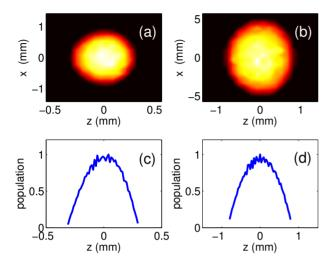
Figure 4: Simulated spatio-temporal distribution (z,x) at s=0.47 m (a) and s=3.77 m (b) (corresponding to X3 screen) wrt to the photocathode and associated longitudinal charge distributions [(c) and (d) respectively]. The charge is 50 pC and the rms laser transverse size is  $\sigma_c=1$  mm. In these plots the tail of the bunch is at z>0.
