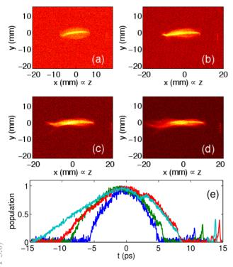
Figure 6: Measured spatio-temporal distribution (z,y) measured at XS3 for four different charges  $130\pm20$  (a),  $280\pm20$  (b),  $461\pm35$  (c) and  $699\pm60$  pC (d) and corresponding normalized current distribution (e) [blue, green, red, cyan traces respectively correspond to images (a), (b), (c) and (d)] . In these plots the tail of the bunch is at (z,t)<0.
