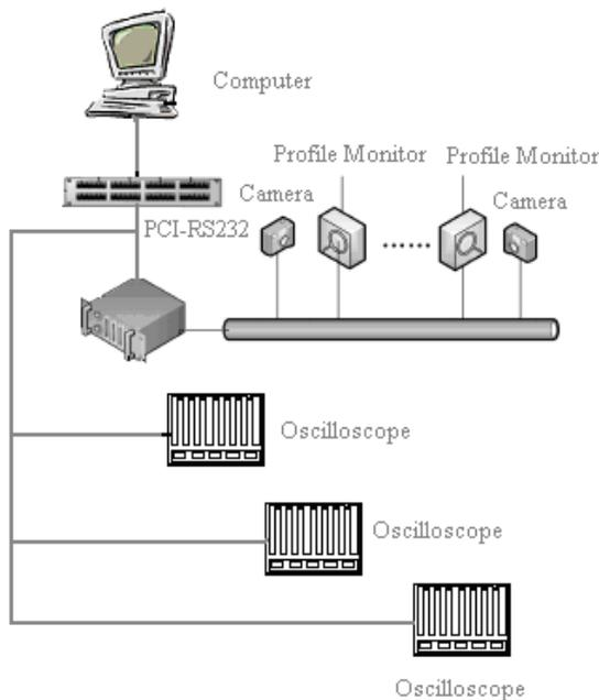
Figure 3: Architecture of Beam diagnostic system
