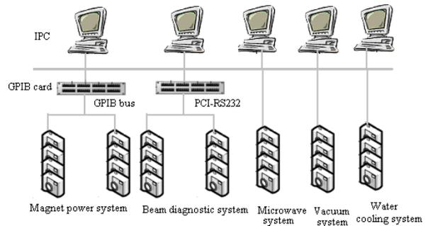
Figure 1: Architecture of the FEL control system
