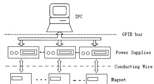
Figure 2: Architecture of the power supply system
