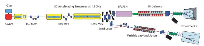
Figure 1: Schematic layout of the FLASH facility. The electron gun is on the left, the experimental hall on the right. Behind the last accelerating module, the beam is switched between FLASH1, which is the present undulator line, and FLASH2, which is the upgrade. Behind the extraction point, space is reserved for an additional laser system for seeding.
