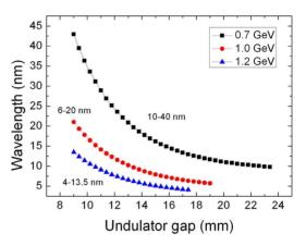
Figure 2: Wavelength range which can be reached for three different energies that are mostly used at FLASH.
