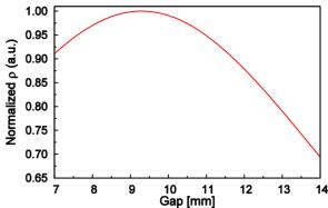
Figure 3: Normalized FEL efficiency vs. the gap of radiator undulators.
