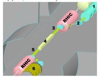
Figure 1: 3-D rendering of the CeC set-up in the RHIC's IP2: 1. 21.8 MeV CW linear accelerator; 2. e-beam transport; 3. CeC modulator section, 4. helical wiggler-FEL amplifier, 5. CeC kicker section, 6. beam dump.
