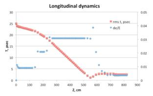
Figure 8: Longitudinal beam dynamics in the CeC accelerator: red dots – e-bunch length in psec, blue – relative energy.y spread (RMS, scale on the right)
