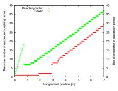
Figure 5: The position of the maxima of optical power (green +) and the bunching factor (red +) with respect to the initial spike, expressed in units of the FEL's wavelength (i.e. 10 µm).
