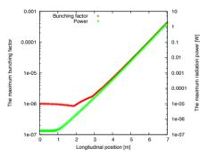
Figure 4: The evolution of optical power (green +) and the bunching factor (red +) by the respective authors/CC BY
