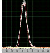
Figure 10: Longitudinal profiles of Au ion bunches in RHIC at 40 GeV/u store.
