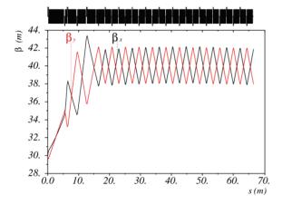
Figure 5: The betatron function in the whole system of the designed HHG-FEL
