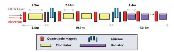
Figure 3: Layout of the hard X-ray HHG-FEL.
