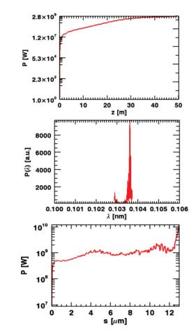
Figure 8: The coherent radiation power, spectral profile and pulse profile by the time dependent simulation.
