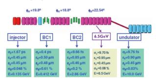
Figure 1: The layout of the linear accelerator that is used by the simulation
