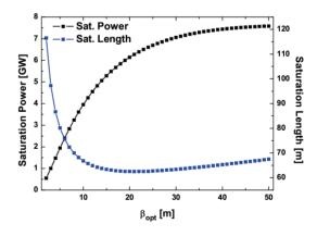
Figure 4: Analytical calculation of the saturation length and power. That are based on the 3-D FEL theory.
