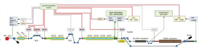
Figure 1: Infrastructure of the laser-based synchronisation system at FLASH. In red all of the seven currently operational fibre links are highlighted.
