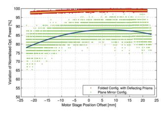
Figure 7: Incoupling efficiency of the new folded configuration compared to the old plane mirror configuration. For a better comparision, the incoupling efficiency is plotted against the offset in motor position not against the optical path length change.
