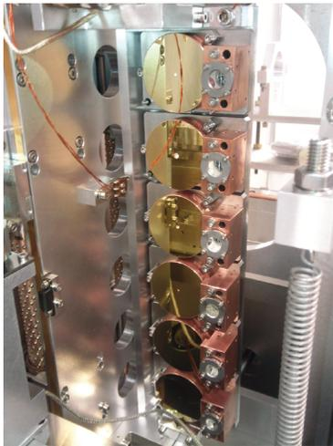
Figure 3: IR cavity mirrors for hole-outcoupling. Gold-plated copper mirrors, with different diameters of the outcoupling hole are mounted on a precision translations stage (design by Bestec GmbH, Berlin). The 50-mm-diameter mirrors have a concave spherical surface of 3.51 m radius of curvature.
