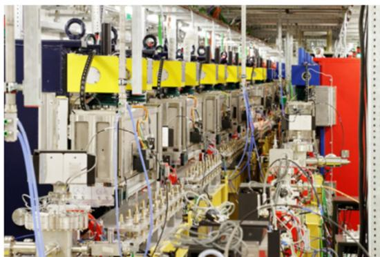
Figure 2: The array of FEL-2 radiators on the left in the picture.
