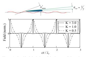
Figure 1: Graphical depiction of the impact of K on the harmonic content of the synchrotron radiation.
