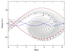
Figure 3: Longitudinal phase space plot of the FEL microbunching including the computed sepratrices for the fundamental (red) and 3<sup>rd</sup> harmonic (blue).
