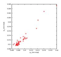
Figure 5: Vertical and horizontal normalized emittance for case with all quadrupoles and sextupoles are random misaligned (Isochronous lattice). For the displacements we used a gaussian distribution with RMS width of 50  $\mu$ m. This represent the worse lattice in term of sensitivity to magnets alignment.
