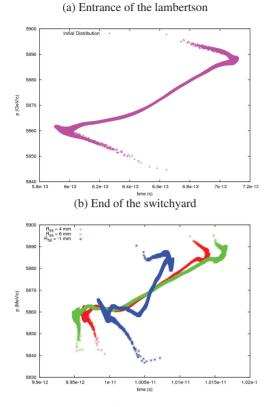
Figure 4: Initial (a) and final longitudinal (b) phase space for different values of  $R_{56}$ . The CSR effects are visible in all cases.
