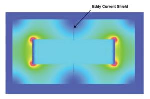
Figure 5: Magnetic field profile of the kicker magnet.
