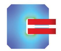
Figure 1: Cross section of dipole magnet (D8) and the field profile.
