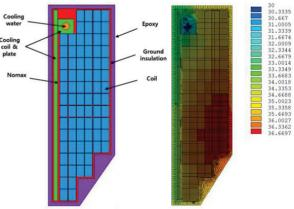
Figure 3: Cross section of quad (Q22-20) coil and the temperature distribution.
