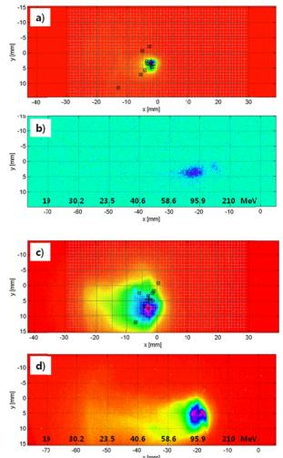
Figure 2: Electron beam position and energy. With parallel nozzle, Electron beam pointing and energy. a) and c) show the electron beam position with parallel and tilted nozzle respectively. b) and d) show the measured electron energy with parallel and tilted nozzle respectively. In a) and c), the circles with cross show the beam position with the same experimental condition.
