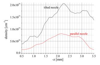
Figure 3: Cross section of the measured plasma density.
