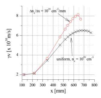
Figure 4: Electron energy in acceleration distance. (2D simulation results.) Open circle shows the electron energy with linearly tapered density and cross shows with parallel nozzle.
