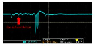
Figure 4: The waveform of PD signal when the self-oscillation occurred.
