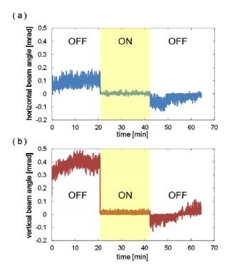
Figure 3: Comparison of the laser beam angle when the regulator was switched on and off, (a) horizontal (b) vertical.
