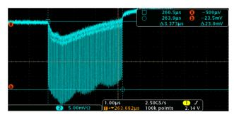
Figure 5: The waveform of PD signal at the amplifier's current value of 80 A.
