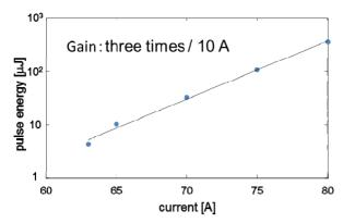
Figure 6: The amplified pulse energy as a function of the LD current.
