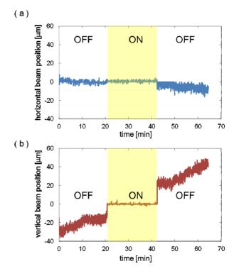
Figure 2: Comparison of the laser beam position when the regulator was switched on and off, (a) horizontal (b) vertical.
