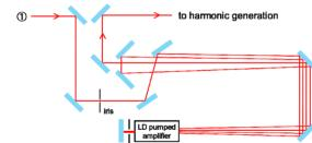
Figure 1: Schematic view of the multi-bunch laser system. (a) shows from the laser oscillator to the beam alignment feedback system and (b) shows a schematic view of the multi-pass amplifier system.
