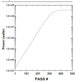
Figure 3: Initial GINGER simulations for output power saturation at the fundamental 13.4-nm wavelength for a concentric cavity with multilayer mirrors and peak current of 800 A at 800 MeV. The output power growth with pass number is shown. (courtesy of M. Reinsch [7])
