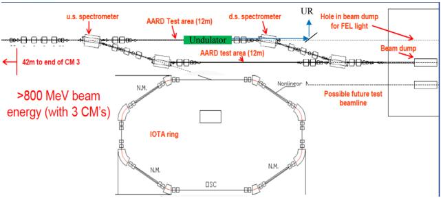
Figure 2: Schematic of the diagnostics undulator located in one high energy test area at ASTA. The output UR is accessed with an in-vacuum mirror/transport after the next dipole. The location of the IOTA ring is also indicated. (courtesy of M. Church, revised).
