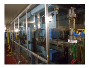
Figure 4: Photograph of the ALS U5.0 Undulator in the storage ring in April 2012. (photo by M. Wendt).
