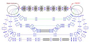
Figure 6: The third stage ERL with FEL undulators.
