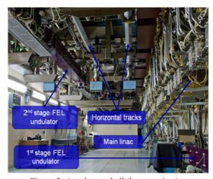
Figure 3: Accelerator hall (bottom view).
