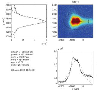
Figure 8: Beam size measurement for the image in Figure 7 representing  $\sim 0.1\%$  energy spread at 45 MeV.
