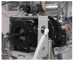
Figure 3: Gridded thermionic gun of the MIR FEL.
