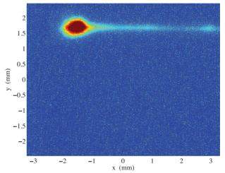
Figure 7: Electron beam image from energy measurement YAG screen in diagnostic beamline.
