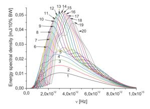
Figure 7: Scan of the dependence on L of the edge radiation pulse energy spectral density transported at the sample position ( $L_s=250$  m downstream of the mirror) as a function of frequency.
