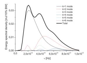
Figure 6: Edge radiation pulse energy spectral density as a function of frequency transported at the sample position.
