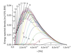
Figure 8: Scan of the dependence on a of the edge radiation pulse energy spectral density transported at the sample position ( $L_s=250$  m downstream of the mirror) as a function of frequency.
