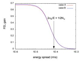
Figure 3: FEL small signal gain as a function of energy spread. The design value is 5E-5 for the case (A) and 1.5E-5 for the case (B).
