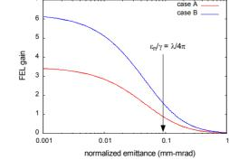
Figure 2: FEL small signal gain as a function of onormalized emittance. The design value is 0.2 mm-mrad.
