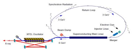
Figure 1: Conceptual layout of the 3-GeV ERL integrated with XFELO at KEK.
