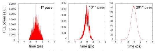
Figure 7: Evolution of a FEL pulse from shot noise to saturation.
