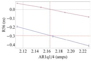
Figure 6:  $R_{56}$  vs. first arc quadrupole strength measured at the exit of the first arc (magenta) and the bunch compressor (blue). The red dotted line indicates the isochronous condition of the first arc.
