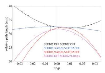
Figure 7: Relative path length vs. energy measured at the exit of the first arc for different arc sextupole (SEXT01 and SEXT02) strengths. Points are measurements, lines are parabolic fits.
