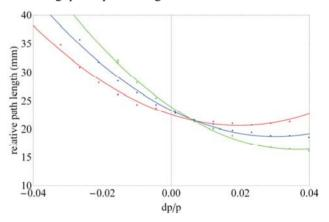
Figure 5: Relative path length vs. beam energy measured at the exit of bunch compressor as the arc quadrupole strengths are varied. Points are measurements, lines are parabolic fits. Red, blue, green, colour sequence represents increasing quadrupole strength.
