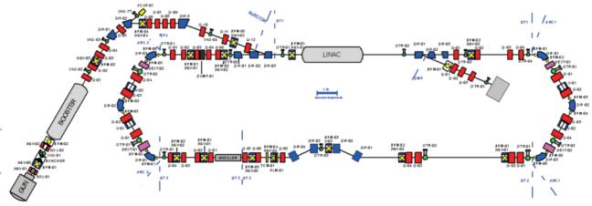
Figure 1: Layout of the ALICE accelerator.
