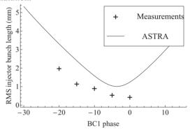
Figure 2: Injector bunch length measurement and simulation as a function of the first booster cavity (BC1) phase.
