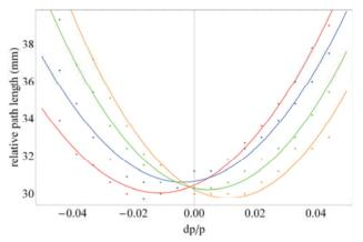
Figure 4: Relative path length vs beam energy measured at the exit of the first arc as the arc quadrupole strengths are varied. Points are measurements, lines are parabolic fits. Red, blue, green, orange colour sequence represents increasing quadrupole strength.
