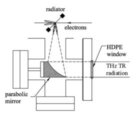
Figure 1: Setup to generate THz Transition radiation.
