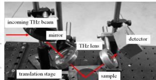
Figure 7: the reflection mode THz imaging setup.
