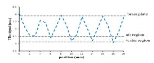
Figure 9: THz-signal line-scan along the dashed line in THz image.
