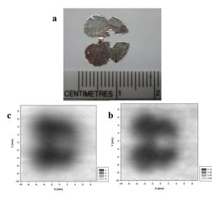
Figure 5: Cut pattern from Al-foil and its THz images; (a) Optical image of the sample, (b) its THz images achieved without mesh filter and (c) its THz image achieved with the mesh filter.
