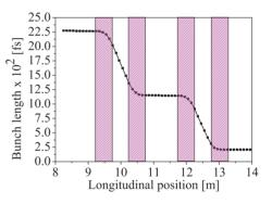
Figure 4: The development of the bunch length tracked through the compressor using ASTRA 3D routines. The shaded parts symbolize the position of the magnets (here 50 cm long).
