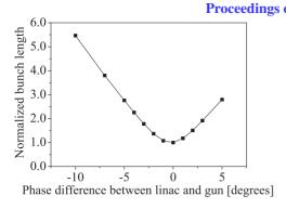
Figure 5: Compressed bunch length as a function of the phase difference between gun and linac cavities calculated with 1D CSRtrack (3 nC charge, 4 ps laser pulse length).
