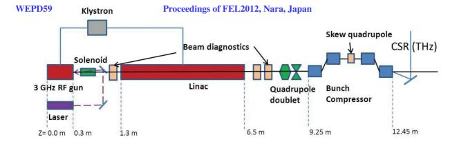
Figure 1: Schematic FLUTE layout (not to scale).
