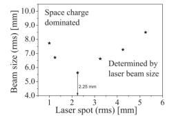
Figure 2: Optimized electron vs laser spot size at the exit of the solenoid after the gun as calculated with ASTRA 3D. For laser spot sizes smaller than 2.25 mm the beam size is increased by space charge effects, for larger spot sizes the beam size is dominated by the laser spot size (bunch charge 3 nC, laser pulse length 4 ps).
