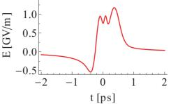
Figure 9: The focused electric field pulse calculated from the 3 nC bunch charge.
