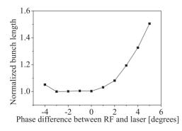
Figure 6: Bunch lengthg as a function of the phase difference between laser pulses and RF signal, calculated with 1D CSRtrack (3 nC, 4 ps laser pulse length).
