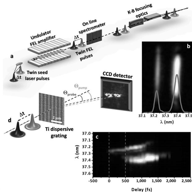
Figure 1: a) Scheme of the generation of the double pulse; b) double pulse as measured by the energy spectrometer; c) sequence of FEL spectra during a temporal scan of the electron bunch-seed laser delay; d) scheme of the experiment.
