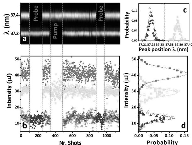
Figure 2: a) Sequence of spectra of both pump and probe as measured by the energy spectrometer; b) intensity of the pulses as measured by both the  $I_0$  monitor and the energy spectrometer used as an intensity detector; c) stability of the peak positions; d) stability of the peak intensities.
