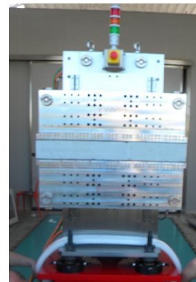
Figure 8: Laser heater undulator.
