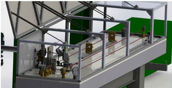
Figure 5: Optical station 0 (OS0). The beam enters from top down to the center mirror in the back. It passes the telescope used for beam shaping and the periscope which is used for XY-alignment, and attenuation system before entering the UHV vacuum. Visible are also the two virtual waistlines used for beam stabilization and analysis.
