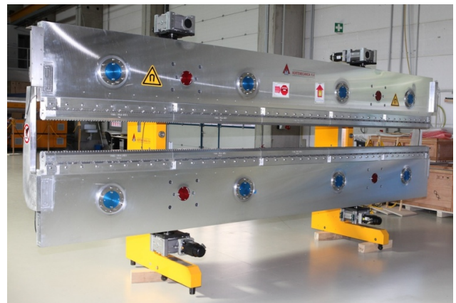
Figure 1: Undulator Segment for SASE1 with \lambda_0=40 mm.
