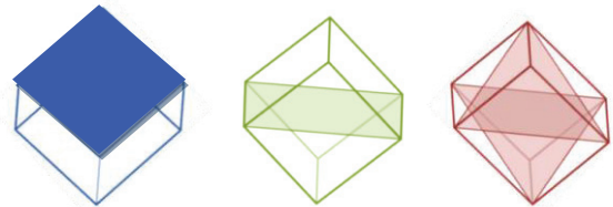
Figure 2: Seeding lines for Bragg reflections with photon energy versus crystal angle for a few basic planes. In blue the [0 0 4] plane corresponds to the surface plane of a cube; its line minimum energy is at 90^\circ (pitch) to the FEL beam. The crystal cube sits then on one of its edges. The [2 2 0] plane cuts diagonally through four corners and its seeding line has a minimum at 0^\circ pitch angle, since its plane would be then 90^\circ to the beam. The [1 1 1] plane cuts through three corners and its perpendicular axis goes through the top, front corner (at 90^\circ pitch). To reach its minimum the pitch angle needs to go further to about 145^\circ . It should be mentioned at this point that with the pitch angle at 90^\circ there are three more corners which have the same angle to the FEL beam and there should be four red lines crossing at the 90^\circ point, the other in-plane line of [-1 -1 1] and the two lines from the out-of-plane planes [-1 1 1] and [1 -1 1] . The perpendicular axes of these out-of-plane planes lie on a cone instead of a plane.
