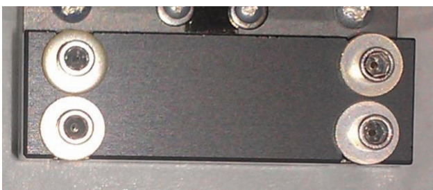
Figure 9: B4C sample after exposure to 1 million pulses of 300 eV x-rays.
