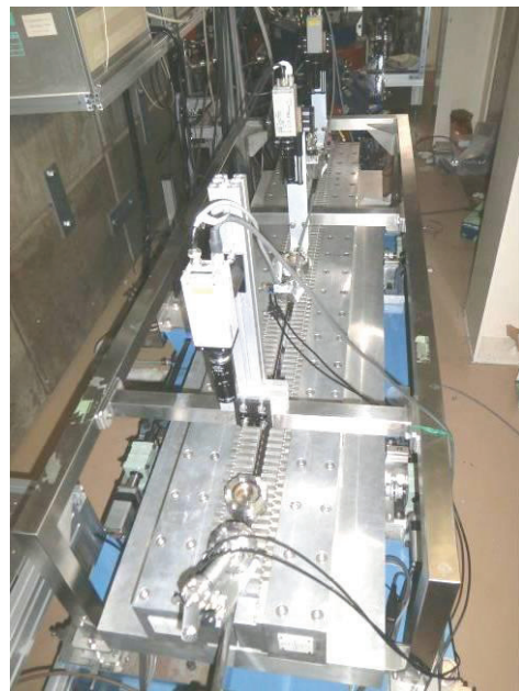
Figure 5: Photo of the undulator with new vacuum chamber.
